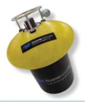
Model R2K Mid-Water Acoustic Transponding Release is a full function acoustic release in a rugged and compact stainless steel housing for use in depths to 2000 meters and loads up to 2000 kg.
